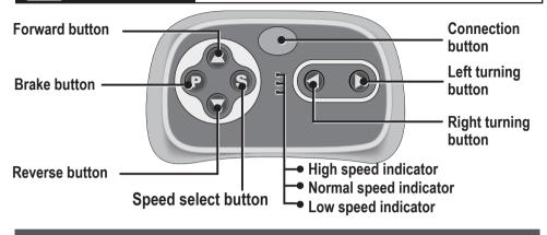
The remote control has precedence over foot pedal operation. (The foot pedal won't work while you operate the Remote Controller)
